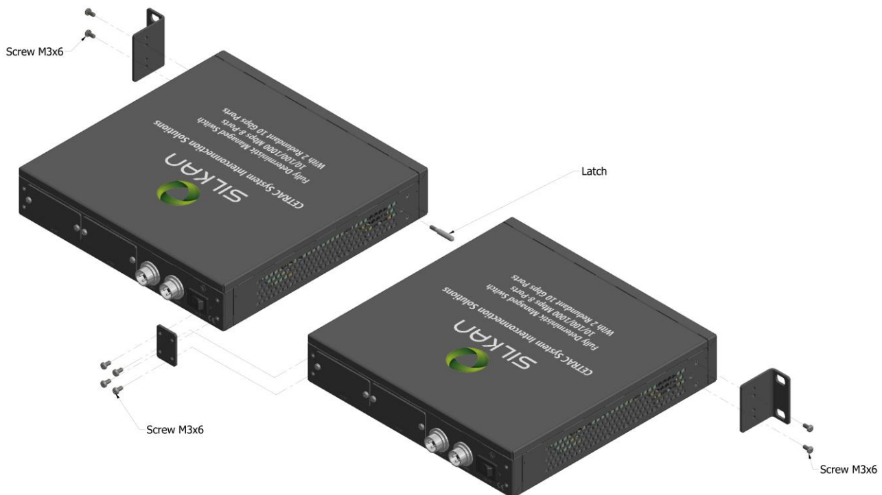
Figure 20 Insertion of 2 CETRAC switches
